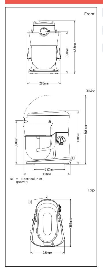
Electric Supply voltage: 200-240 V/1N ph/50/60 Hz **Total Watts:** 0.5 kW Capacity: Performance (up to): 0.75 kg/Cycle Capacity: 5.5 litres Key Information: External dimensions, Width: 280 mm External dimensions, 388 mm Depth: External dimensions, Height: 438 mm 15 kg **Shipping weight:** Net weight (kg): ISO 9001; ISO 14001 0.75 kg with Semi spiral **Cold water paste:** hook
